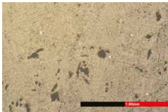
FIGURE 7 BRAD 1007 3, moderate fine wüstite dendrites and metallic prills
